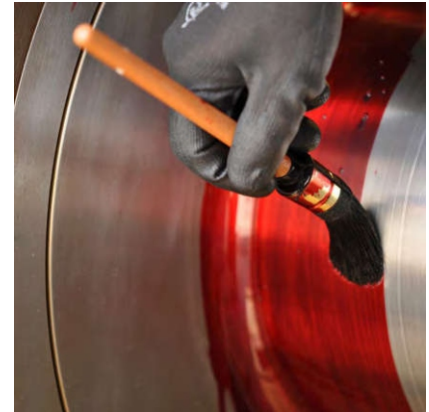
DYE PENETRANT TESTING
