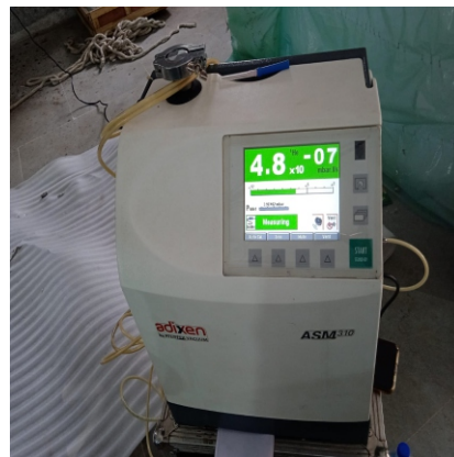
FUGITIVE EMISSION TEST
